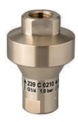
The EcoReg<sup>®</sup> fluid regulator is an independent diaphragm pressure regulator that can be installed in all fluid systems. The pressure regulator ensures a constant and precise output pressure independent from the input pressure. The pressure value has been factory preset and cannot be changed. This ensures that no one can manipulate the specified pressure value.
