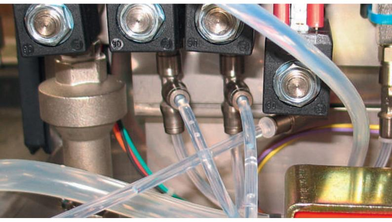
The FluidReg<sup>®</sup> is an independent diaphragm regulator that can be installed in every fluid- or compressed air pneumatic system. It supplies a constant, exact outlet pressure regardless of the input pressure. The pressure is factory-set and cannot be changed. This ensures that nobody can alter the specified pressure.
