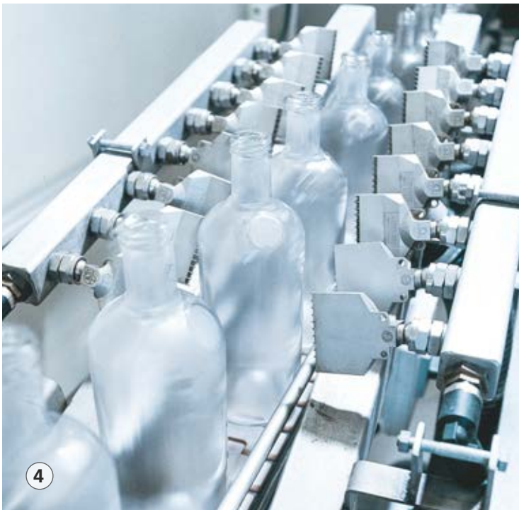
Drying with SILVENT 973 nozzles for better quality.
