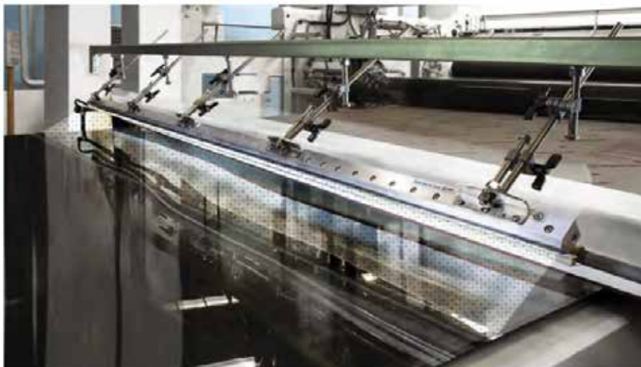
This 96" Long Super Ion Air Knife cleaning an acrylic sheet before protective wrap is applied.
