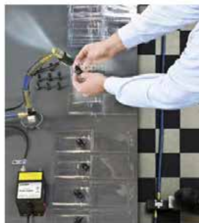
The Model 8910 Instant Static Elimination Station removes contaminants on plastic clamshell packages.
