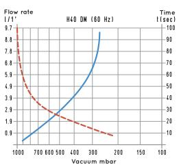
To calculate the emptying time of a volume of  $V_1$ , use the following formula:  $t_1 = \frac{t \times V_1}{6}$
