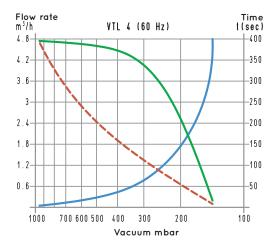
**t x V**<sub>1</sub> To calculate the emptying time of a volume of  $V_1$ , use the following formula:  $t_1 = -$ 100 Curve relative to the flow rate (referring to the suction pressure)
