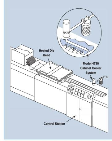
**The Problem:** In the pultrusion process, resin coated fibers are assembled by a forming guide, then drawn through a heated die. Residual heat from the die caused electronic malfunctions at the control station located immediately downstream.
