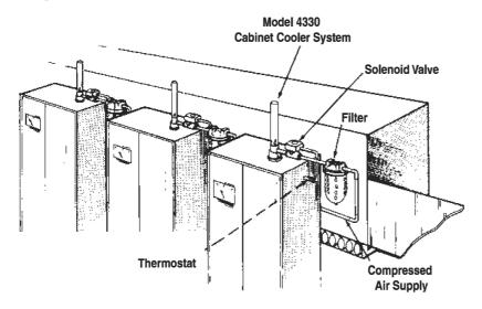
**The Problem:** Few companies contend with more heat-related problems than do glass manufacturers. Control panels in close proximity to molten glass are particularly susceptible. High ambient temperatures caused constant "nuisance tripping" of the circuit breakers. The "quick fix" solution — opening the panel doors — allowed dirt to enter the panels and created a potential safety hazard.
