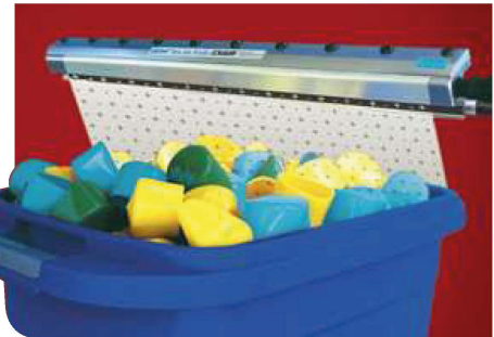
The Model 8218 18" (457mm) Gen4 Standard Ion Air Knife System showers parts with static eliminating ions to prevent personnel shocks.
