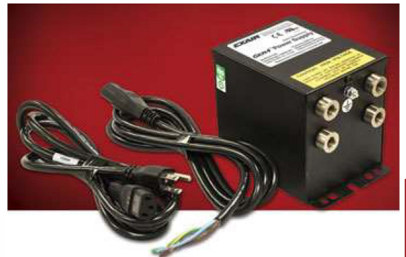
The Model 7961 Gen4 Power Supply has 115VAC or 230VAC selectable voltage, lighted power switch, integral fuse on the primary, electromagnetically shielded modular power cable and (4) 5kV outlets.
