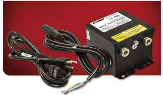
The Model 7960 Gen4 Power Supply has 115VAC or 230VAC selectable voltage, lighted power switch, integral fuse on the primary, electromagnetically shielded modular power cable and (2) 5kV outlets.
