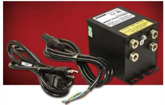
The Model 7961 Gen4 Power Supply has 115VAC or 230VAC selectable voltage, lighted power switch, integral fuse on the primary, electromagnetically shielded modular power cable and (4) 5kV outlets.
