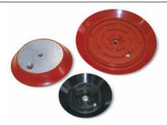
These cups have been designed for lifting and handling heavy loads, both vertically and horizontally. They are vulcanised onto a steel support and are provided with a central threaded hole for its fastening to the machine and with a side threaded hole for vacuum connection.
