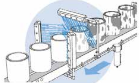
(3) Model 110012 12" (305mm) Super Air Knives blow excess honing oil off machined engine sleeves.
