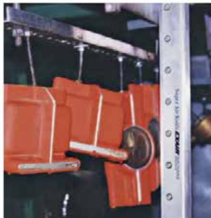
A Model 110018 18" (457mm) Super Air Knife cools molten plastic following dip molding.
