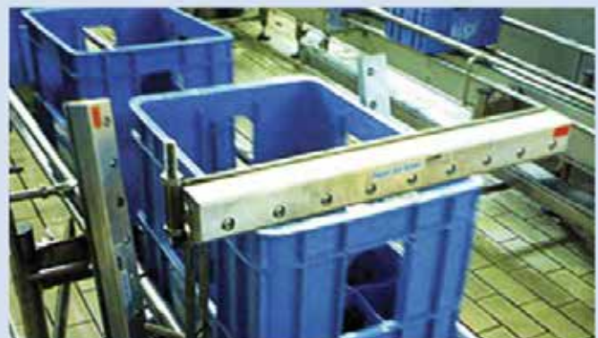
Three Model 110018 18” (457mm) Super Air Knives completely surround and blowoff crates so they can be loaded immediately.
