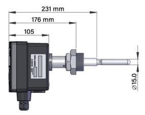
PROBE ROD LENGTH 300mm | 600mm | 1000mm **ORDERING CODES** Please note that along with the PEM code you must always order either the P300, P600 or P1000 (respectively for the 300 mm long rod, the 600 mm long rod and the 1000 mm long rod) Imperial temperatures given are nominal values
