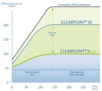
The operating costs for the CLEARPOINT® 3eco filter can be considerably lowered. The graphic illustrates them on an example of the S040 filter with filter ration S with energy-optimised volume flow.
