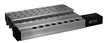
Sub-bases with fix position for A2 series valves, with standard 25 poles SUB-D connector, can be mounted on DIN EN 50 035 guides.
