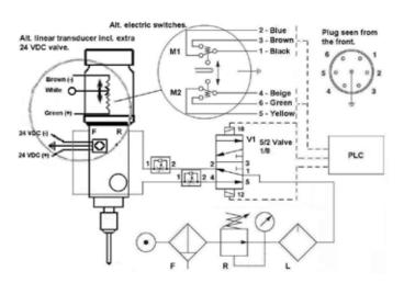
The max load for the switches at 220 V is 1A.
