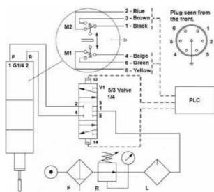
The max load for the switches at 220 V is 1A.
