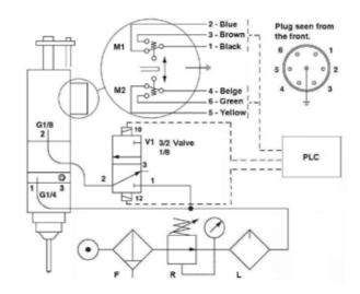
The max load for the switches at 220 V is 1A.
