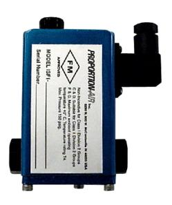
Hazardous media such as natural gas can be directly controlled with the ISF1 Nonincindive-Factory Mutual (Class II, Division 2 Groups C, D) electro-pneumatic closed loop pressure control valve. Offered with standard 4-20 mA analog command signal and 13.5 to 29 VDC supply voltage. Can be assembled to air piloted regulator for high flow, higher pressures and various media control.
