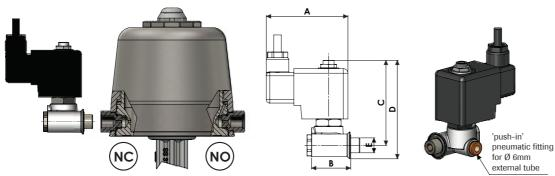
Screw the pilot valve bolt into the inlet port of the piston valve actuator using a maximum torque level of 5 Nm:
