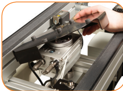
STANDARD FEATURE: Breakaway Top Plate
